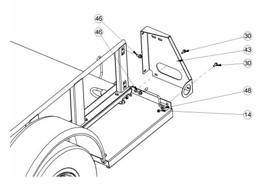
Position Rear Fender Braces (Item 43) on either side of trailer as shown. Bolt Fender Brace and Side rail together with 3/8" Flange Bolt (Item 46). Bolt Fender Brace and Rear Fender together with 5/16" Flange bolt, washer and nut (Items 30, 48, 14).
