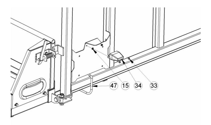
• Install License Plate Light (Item 34) as shown on License Plate Bracket with the light shining down on license plate area.
