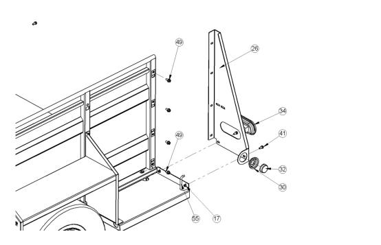
Install High Wall End Caps (Item 26) with 3/8" Flange Bolts (Item 49) into side wall J-Clips. Use 5/16" Flange Bolts and Nylock nuts (Items 41, 17) to bolt End Cap to Bolt-On Fender. • Connect Wiring Harness (Item 55) to Tail Lamp and Side Marker Light.
