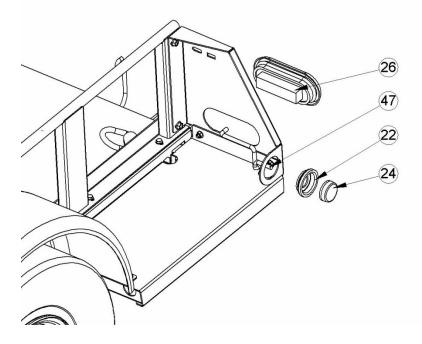
• Install Tail Light (Item 26) and Red Side Marker Light (Item 24) in Rear Fender Brace as shown. Plug Wiring Harness connectors (Item 47) into the lights.
