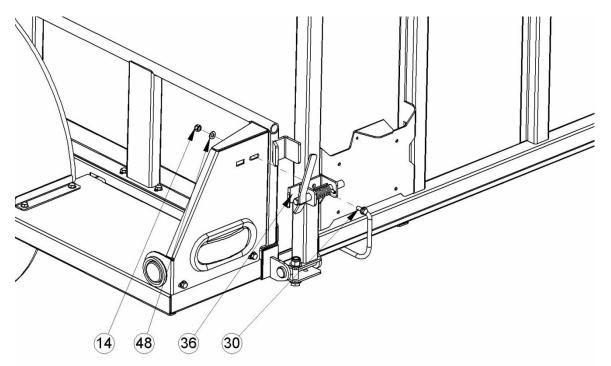
• Install Ramp Latch (Item 36) onto Fender Brace in locked position as shown. Slide Ramp Latch in slots until Lock Pin and Ramp Catch Plate are overlapped 5/8"-3/4". This will ensure proper function of Ramp Latch.
