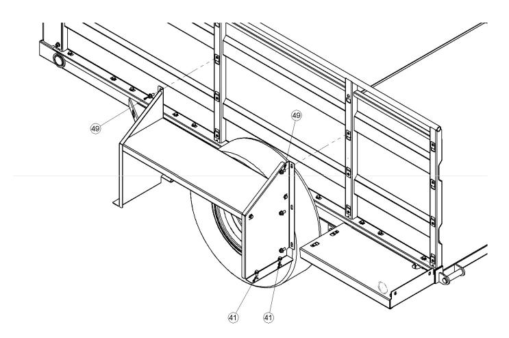
Install both Fender Assemblies as shown with 3/8" Flange Bolts (item 49) into side wall J-Clips and 5/16" Flange Bolts (Item 41) into the Bolt-On Fender J-Clips.
