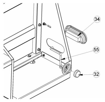
• Tighten ALL side wall bolts, corner brace bolts and fender bolts at this time.
