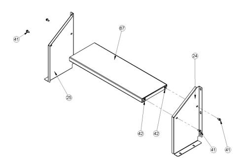
Assemble both Side Fenders as shown. Install 5/16" J-Clip Nuts (Item 42) in either end of fender (item 67). Bolt together Fender Assembly with 5/16" Flange Bolts (Item 41).
