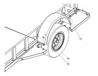
• Install fenders (Item 40) on either side with 5/16" Flange Bolts (Item 30). Tighten bolts.
