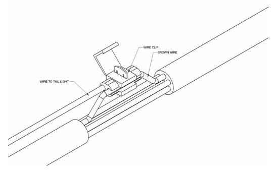
The License Plate light will have a length of wire connected to it. Route this wire back under the trailer to the Side Marker/Tail Light wiring. Splice License Plate wiring into Tail Light wiring with the provided Wire Clip as shown.
