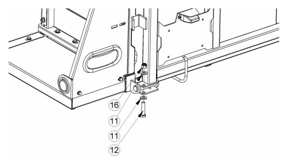
Place Ramp Section onto ramp pivots at the back of the deck. Rotate ramp into vertical position and install ½" bolt, washers and nylock nuts (Items 12, 11, 16). Bolts MUST be installed as shown to ensure proper function of Ramp.
