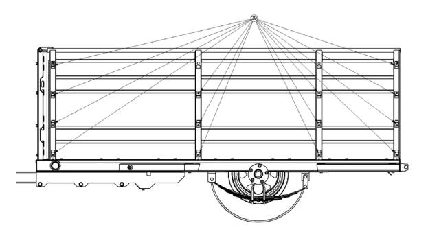
• Prepare the High Side and Front Wall sections for assembly by installing 3/8" J-Clip Nuts (Item 29) in the side rails as shown.
