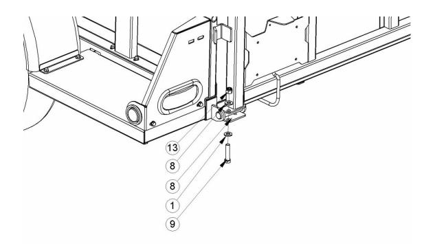
Position Ramp Section (Item 1) onto Trailer Deck and pivot up into upright position as shown. Install ½" Bolt, Washers and Nut. Tighten Nut until Bolt is tight but does not clamp down on pivot shaft. Bolts must be installed as shown for proper function.
