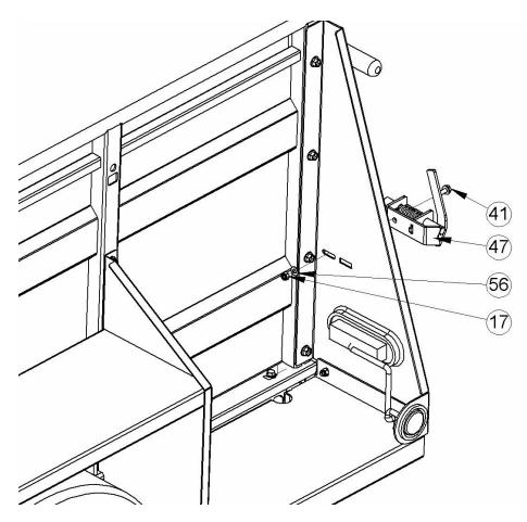
• Locate Ramp Latch (Items 47, 48) and install on either side as shown. Position Ramp Latch Pin in the locked position overlapped 5/8"-3/4" with ramp plate as shown, tighten flange bolt and nut.
